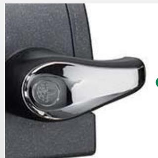
**2 C-LEVER** (Rancilio Patent) The new steam valve with a special control knob and ergonomic design is complete with open-stay and open-close functions. The valve has a very short travel distance, and is operated by rotating it just 25°. Turning it upwards, it opens and remains in this position. Turned downwards, it automatically closes when released. Rapidity, precision and ergonomics: maximum user comfort for daily tasks.
